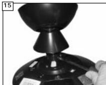
Tighten set screws to hold downrod securely in the yoke. Drop cover over yoke.
